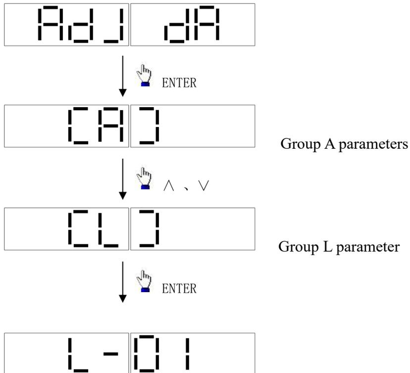
( If no operation is performed, the value of this parameter is displayed one second later. The other parameters are the same )
