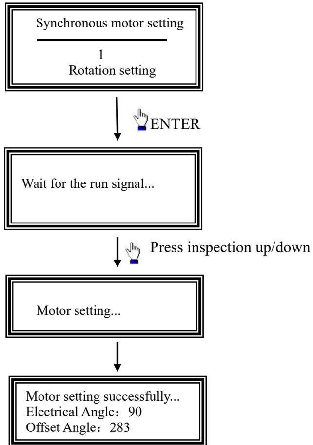
8.If cannot release load (when there is no hanging wire rope), the setting mode is set to 1, and the stationary synchronous motor self-learning is performed
