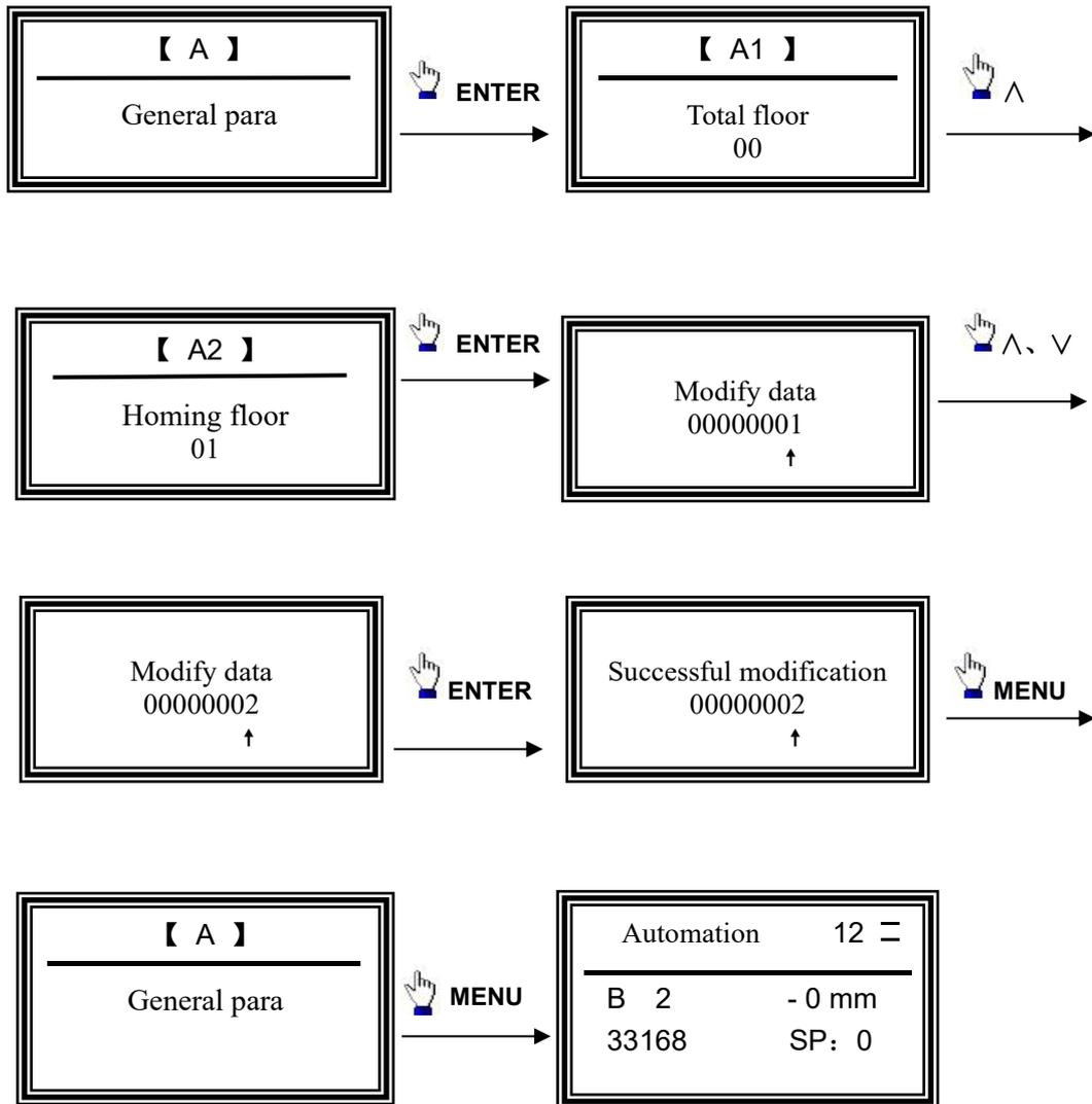
Note: Most of these operations are in parameter menu. Press menu key to exit the menu, press ^ and v key to flip the menu and add or subtract operation data, press > key to move cursor, press ENTER key to select function or confirm data.
