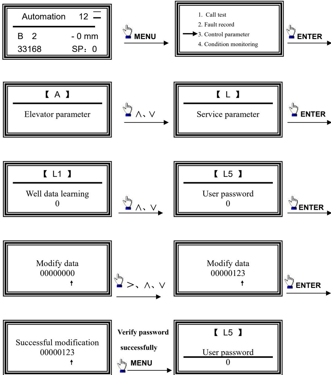
**4.5.2 Parameter Adjustment Menu Common functions: A2 parameter - Waiting base station (for password input, see the previous description)**
