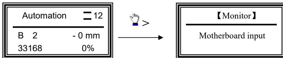
The menu of state monitoring has 9 submenus, which are: main board input], outgoing call communication, internal call registration, upcall registration, downcall registration, car input, car output, current and voltage, data monitoring. Switching between each submenu and monitor page presses "^" "v" key. Entering the submenu presses "Enter" key. After entering the submenus, press MENU to return, and then press MENU to return to the initialization screen.
