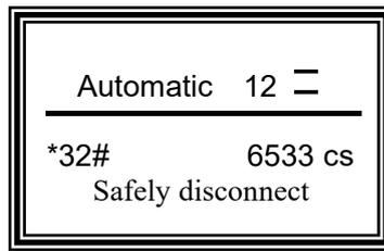
If an elevator fault occurs during operation, the fault will be displayed on the bottom line of the LCD screen. So you need to press ENTER to eliminate the fault. If the fault persists, rectify the fault.
