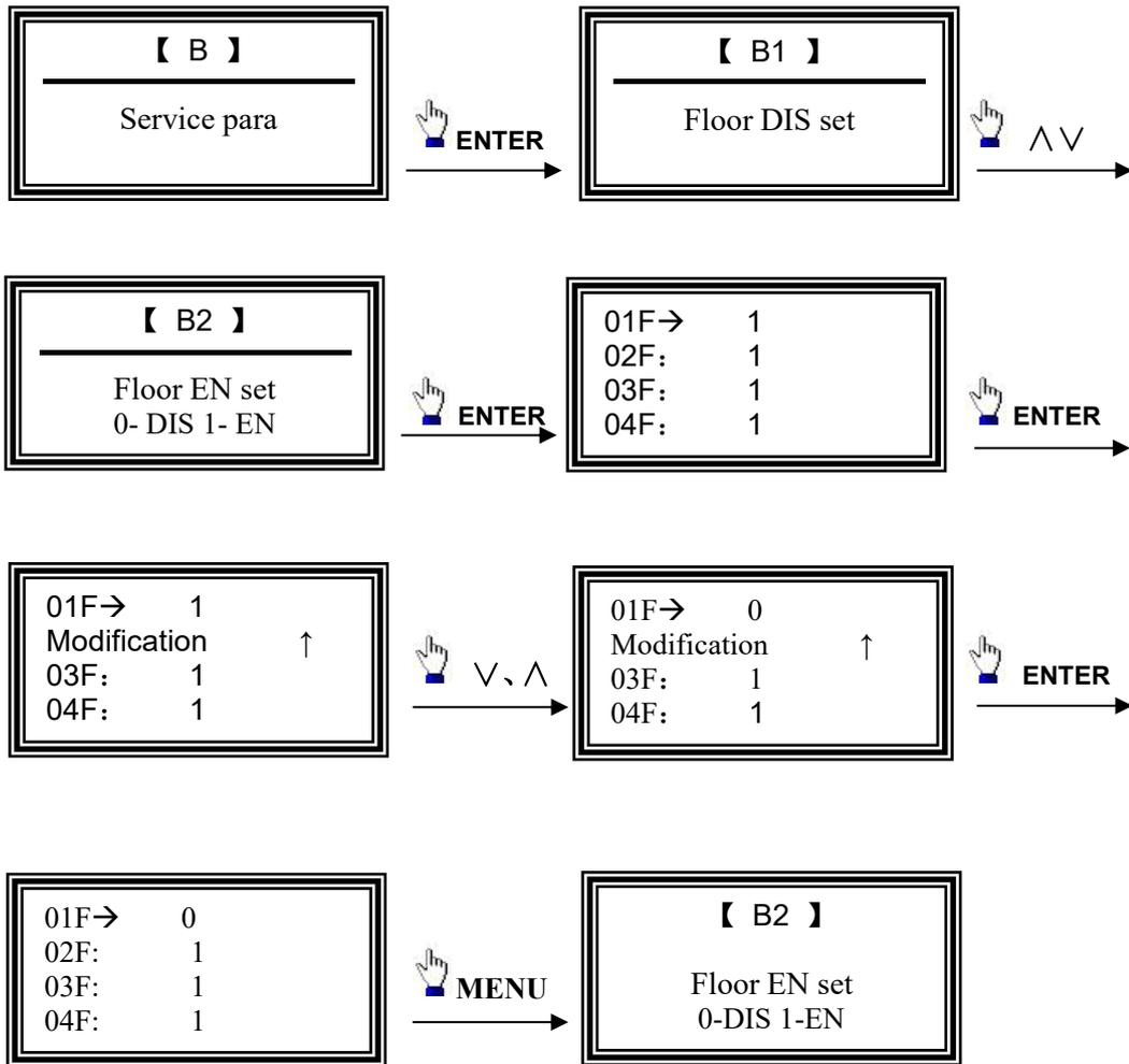
Note: In this class MENU, press menu key to exit the menu, press **^**, **v** key to move cursor, press **>** key to function And data transformation or page turning, press **ENTER** key to select the function or data confirmation.
