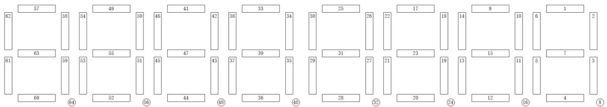
If the input point X1 has a signal input, the corresponding dot is lit.
