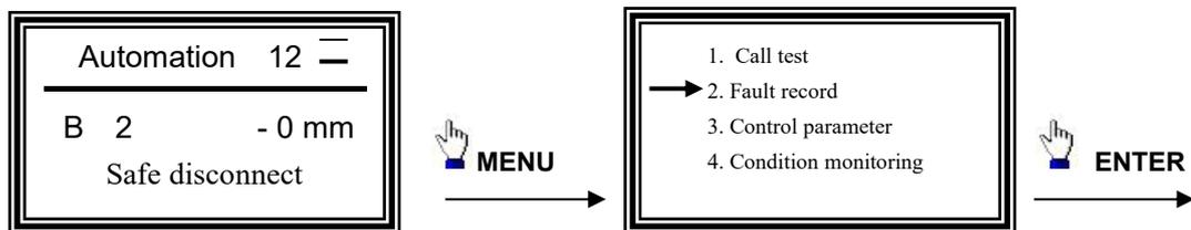
Note: If the elevator fails during operation, the current fault name will be displayed in the bottom line of the LCD operator. After the fault is removed, press "ENTER" to eliminate the fault display. If it cannot be eliminated, it means that the fault has always existed
