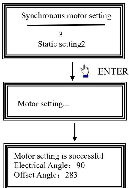
9. After the complete setting mode 1 (rotation) or setting mode 3 (stationary) is successfully performed, the elevator can be repaired normally. If debugging personnel think that the encoder signal is not accurate in the field, they can learn the setting mode 4 again, so that the encoder Angle learning is more accurate. After the learning of the setting mode 4, they should learn the setting mode 1 or setting mode 3 again.
