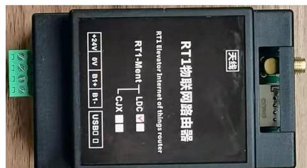
1. The SIM card slot can accommodate a SIM mobile phone card with a 13\*\*\*\*\* card number (the phone card chip faces down, the notch faces outward, be careful not to insert it incorrectly).
