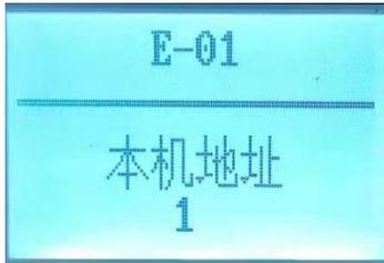
Single Elevator: (Set the 1st elevator as 01, the 2nd elevator as 02.)
