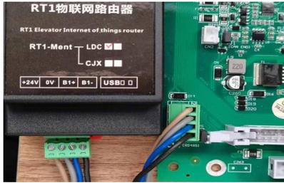
5. Set the elevator number in the E01 parameters of the LDC100BCN mainboard:
