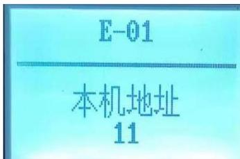
Group Control: (Set the 1st elevator as 11, the 2nd elevator as 12, the 3rd elevator as 13....)
